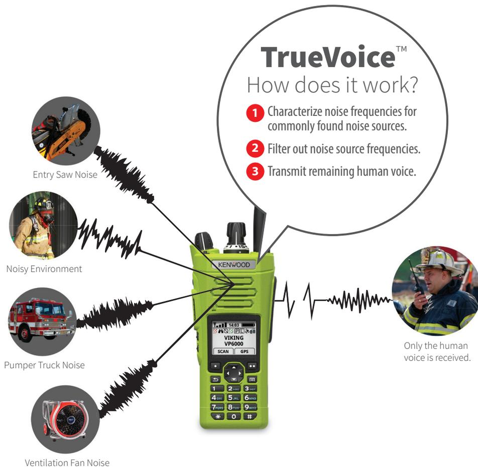
The illustration below demonstrates the comparison between the dual microphone and TrueVoice products. Dual microphones lower and degrade the first responder's audio, whereas TrueVoice retains the audio level and intelligibility.
