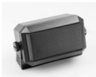
**Details:** 10W 4 Ohm External Speaker with 3.5 mm audio plug. General Specifications: Housing: Black plastic ABS. Dimensions 110.0 (W) x 66.0 (H) x 55.0 (D) mm. Height with retaining bracket is 77.0 mm. Connection: 2-wire cable 3.00 m, with 3.5 mm phone jack. Temp Range: -13°F to +158°F (-25°C to +70°C). Output: rated 10W / max. 12 W. Impedance: 4 Ohms ± 15% (at 600 Hz). Frequency Range: 300 Hz to 7 kHz at -10 dB. Total Weight: 385g.
